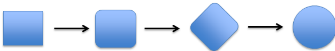
Figure 37: Theoretical figure for the transition of square water drop into steady state as a circle
